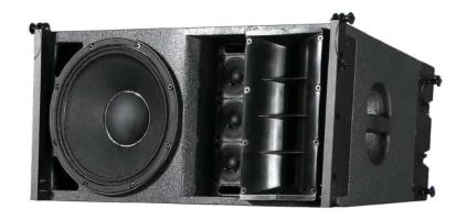
HDLA8055 V2 is a line array loudspeaker for large scale sound reinforcement, fitted with 1x12" Neodymium LF driver, 3x3" Neodymium MF drivers and 2x1" Neodymium HF driver with line array horn, made of high quality plywood with polyurea waterproof paint. All rigging parts are made of aluminium alloy.
